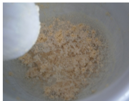
Figure SM 4.2.2.3.1 – Reaction mixture: a) paste at the beginning of the grinding; b) using the spatula to remove the solid from mortar's wall; c) beige solid obtained after complete grinding.
