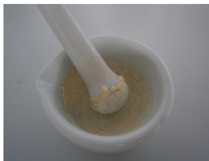
Figure SM 4.2.2.3.1 – Reaction mixture: a) paste at the beginning of the grinding; b) using the spatula to remove the solid from mortar's wall; c) beige solid obtained after complete grinding.
