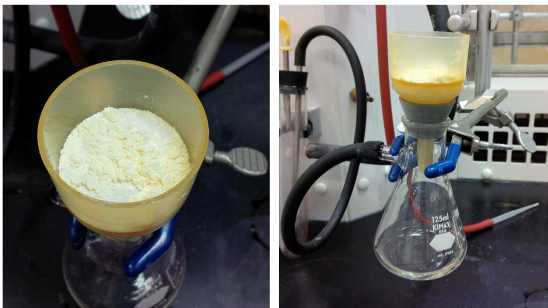
Figure SM 4.2.2.1.2 – Collection of the crude solid by suction filtration on a Büchner funnel.
