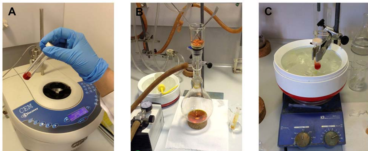
Figure SM 4.2.2.9.1. Different phases of the experiment. (A) Reaction mixture of the enaminone synthesis after microwave irradiation. (B) Filtration of the enaminone after crystallisation in toluene. (C) Reaction mixture of the chromone synthesis before microwave irradiation.
