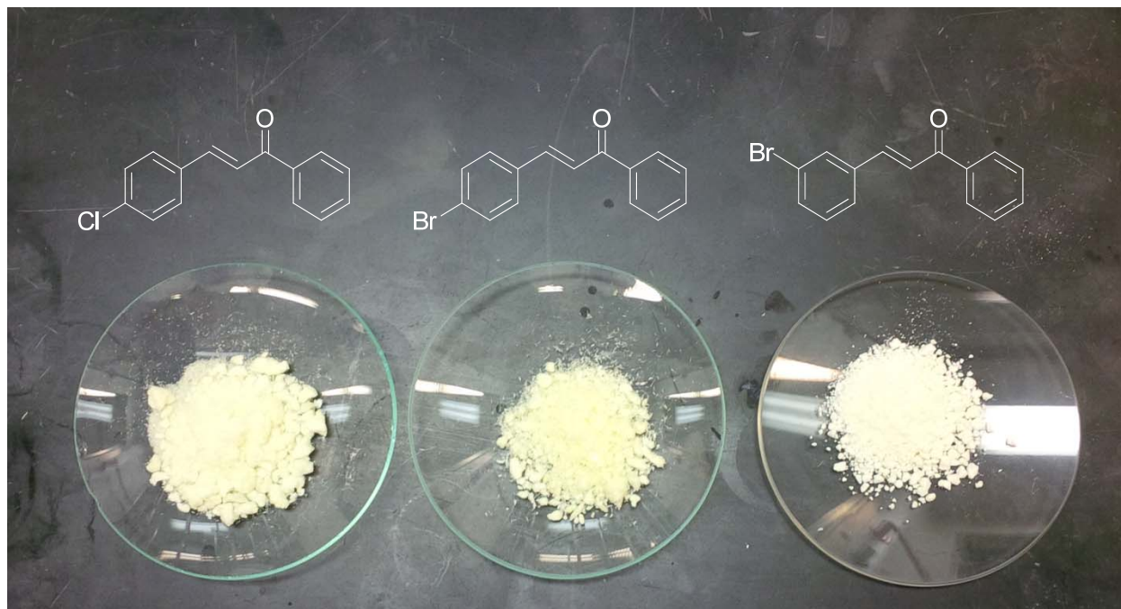
Figure SM 4.2.2.1.3 – Pure chalcone products after recrystallization (all pale yellow crystals).
