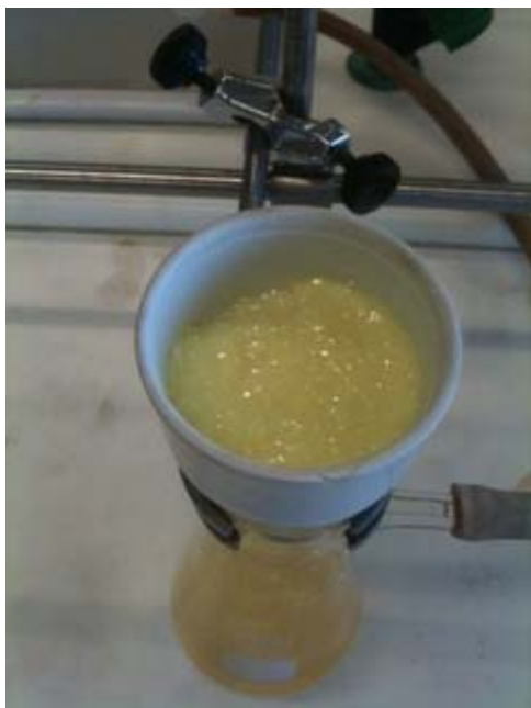
Figure 4.2.2.4.9. Collecting crystals by suction filtration Figure 4.2.2.4. 10. Crystals of purified product
