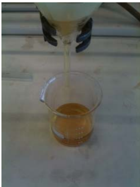
Figure 4.2.2.4.7. Hot filtration after recrystallization
