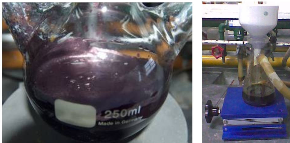
Figure SM 4.2.2.10.1 – Indigo after precipitation and vacuum filtration
